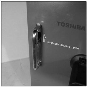
Fig. 3 Interlock Release Lever
